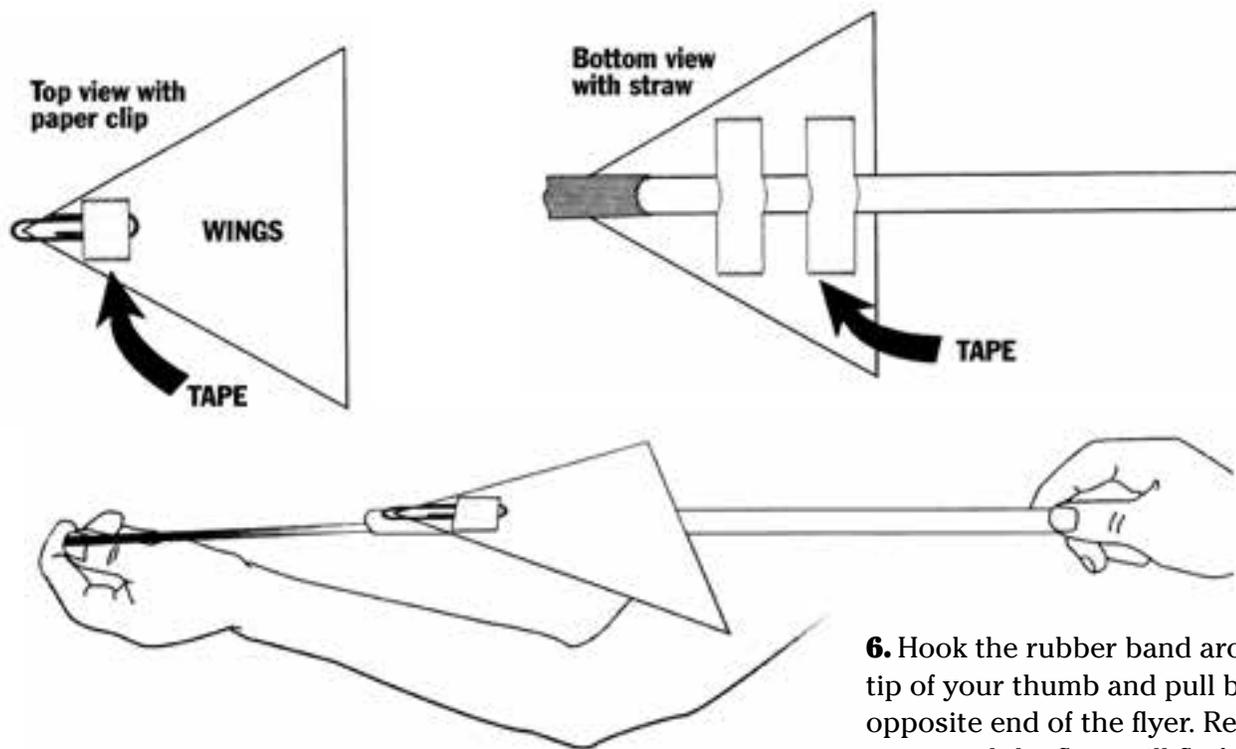
6. Hook the rubber band around the tip of your thumb and pull back on the opposite end of the flyer. Release the straw and the flyer will fly forward.
