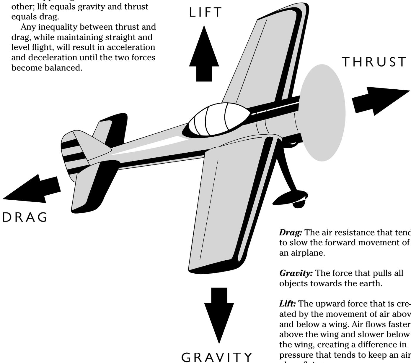
**Drag:** The air resistance that tends to slow the forward movement of an airplane.
